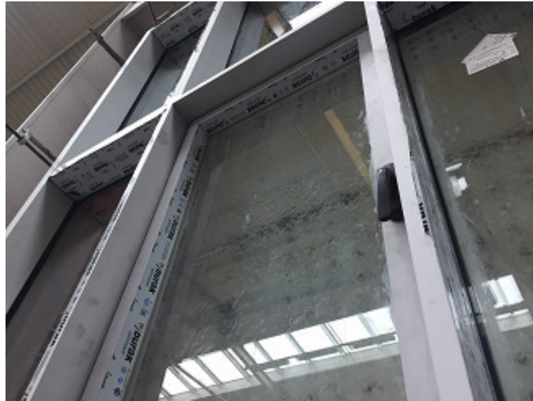
Photo 02. A view of the specimen while watertightness testing
